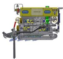
QT1500 ROV system is newly supplied by SMD, and is track & free swimming type ROV for cable & pipes up to 1,000m water depth. Maximum burial depth achievable is 3.0m (subject to soil conditions) with 1,500HP of power and QT1500 ROV trenches down telecom & power cables, as well as small diameter pipelines.
